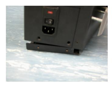
As shown in the picture, use 4 screws to attach the dock assembly. Check the alignment as described on page 5. Shims may be needed in front or rear of the bracket (between the bracket and the mat) to make sure the dock does not tip forward or back.
