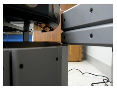
As shown in the photo, the plates of the charging dock must line up with the robot's front contact bezel. It is important the the bottom plate does not hit the front bumper but rather naturally rides up on the robot's bottom platform. As the robot pushes further into the dock, the top charging target
